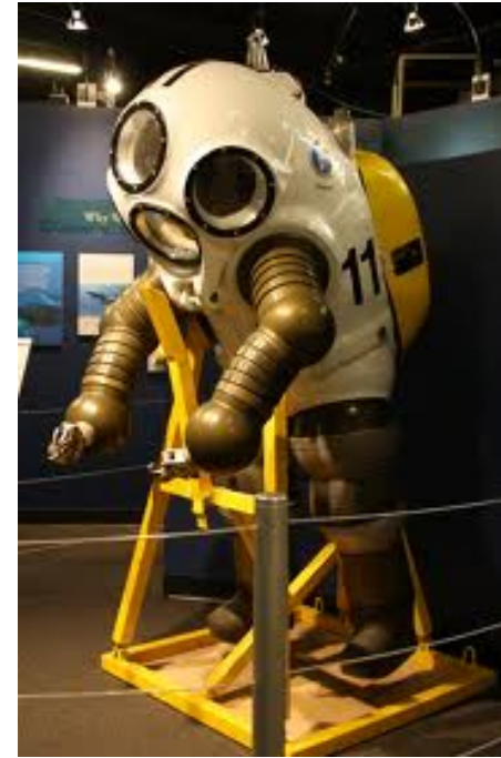
Atmospheric Diving Suit up to 600 m underwater
